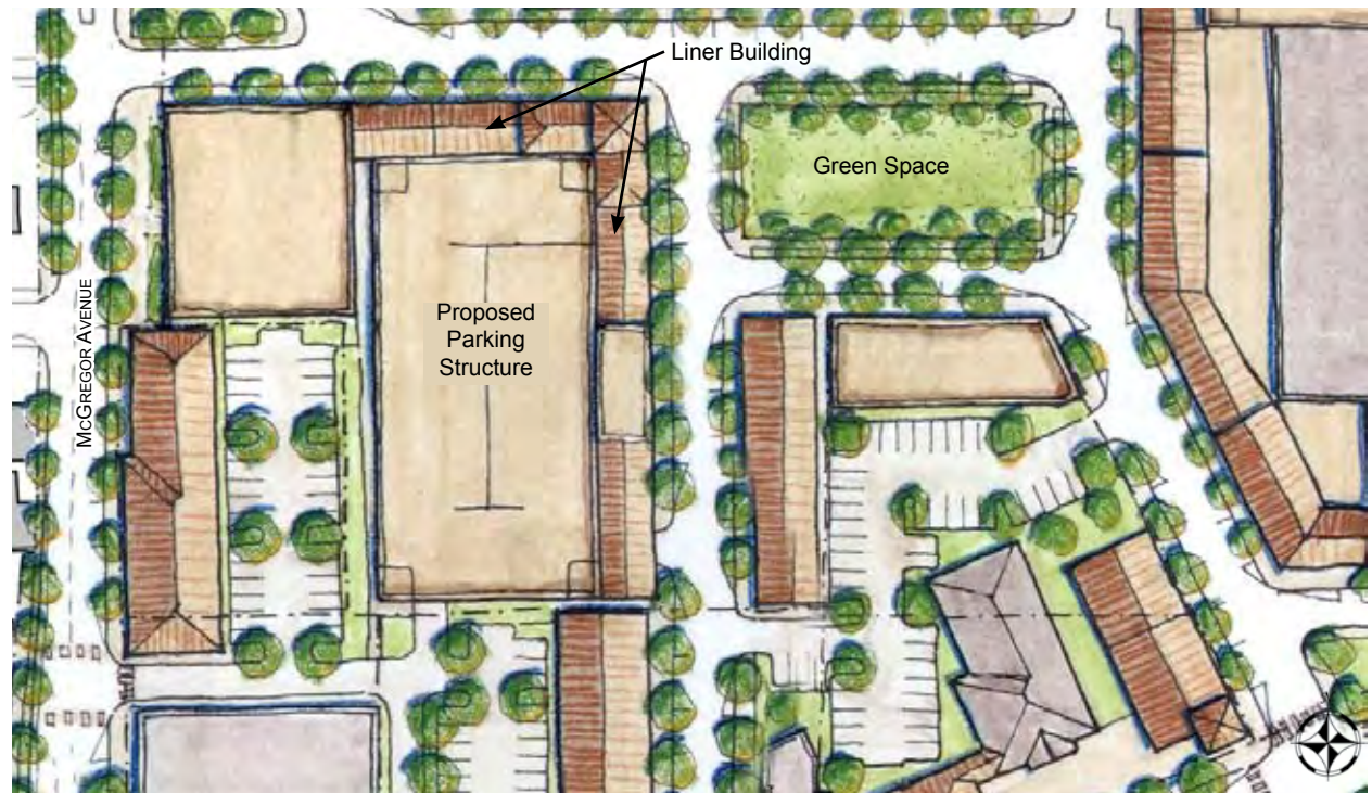
A lined parking structure absorbs surface parking allowing additional development and green space.
