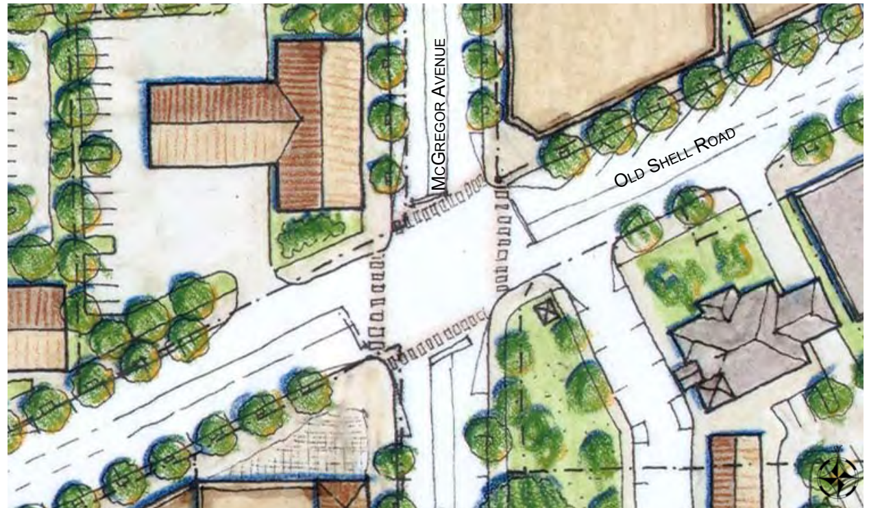
Proposed revisions to the intersection of Old Shell Road and McGregor Avenue include eliminating the right turn lane (creating a shorter crossing distance for pedestrians), and adding on-street parking, defined crosswalks, wider sidewalks, and new street trees.
