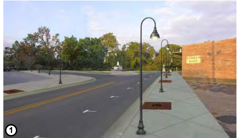
Step 1: Public improvements set the stage for a walkable neighborhood center. Overhead utility lines are removed, generous sidewalks are built, pedestrian-scaled lighting is provided, and on-street parking, a new safer intersection, and a neighborhood green are implemented.
